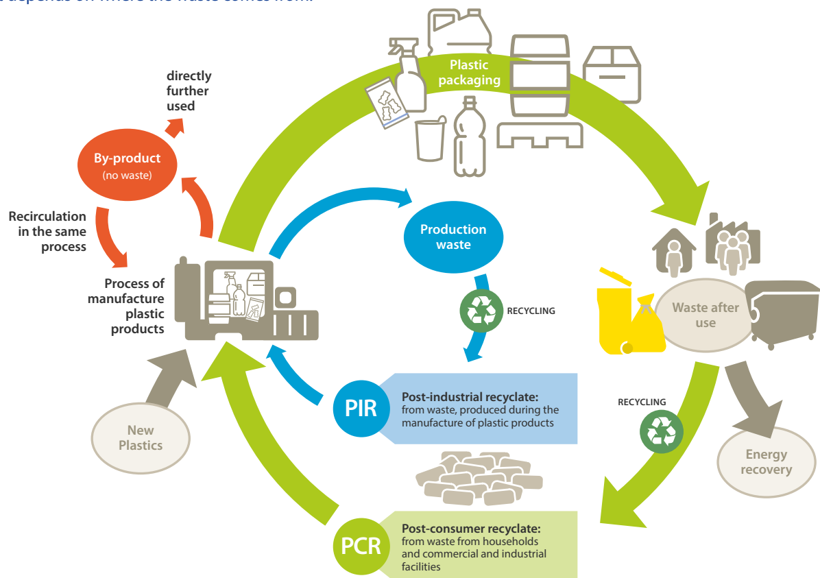
Figure 6: Difference between post-consumer recycle and post-industrial recycle: The decisive factor is where the recycled plastics come from.
